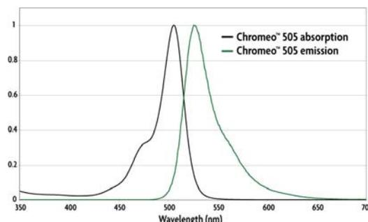
**Absorption and emission spectra of Chromeo 505 Dye.**
