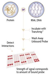
Figure 1: Flow chart of the TransArray process.
